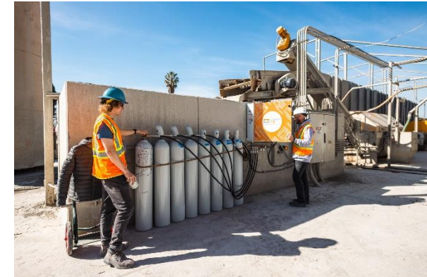
Inject CO 2 into fresh concrete, where it converts to a solid mineral, calcium carbonate (CaCO 3 ) (e.g. CarbonCure®).
